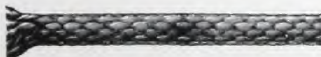
SIZE NO. 7. DIAM. 7-32 IN. About 22 lbs. per doz.; about 55 ft. per lb. Suitable for weights from 5 to 12 lbs. Minimum diam. of pulley allowable, 1 3/4 in.
