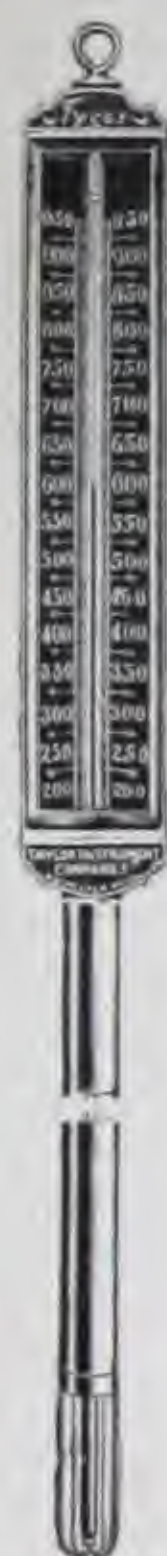
TYCOS INDICATING THERMOMETER FOR STACK TEMPERATURES.
