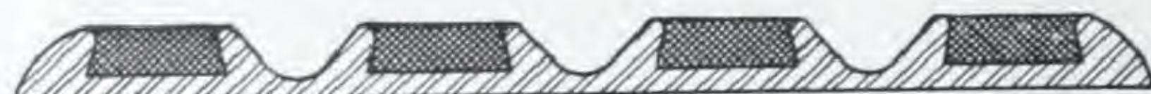
Fig. 3A. Cross Section, steel, 4 ribs, 3 3/4 inches wide.
