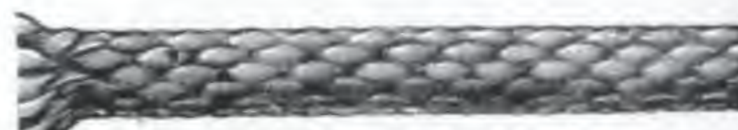
SIZE NO. 9. DIAM. 9-32 IN. About 33 lbs. per doz.; about 36 ft. per lb. Suitable for weights from 20 to 30 lbs. Minimum diam. of pulley allowable, 2 1/4 in.
