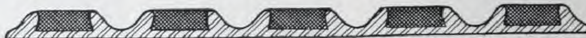
Fig. 2. Cross Sections, steel, 5 ribs, 4 1/4 inches wide.
