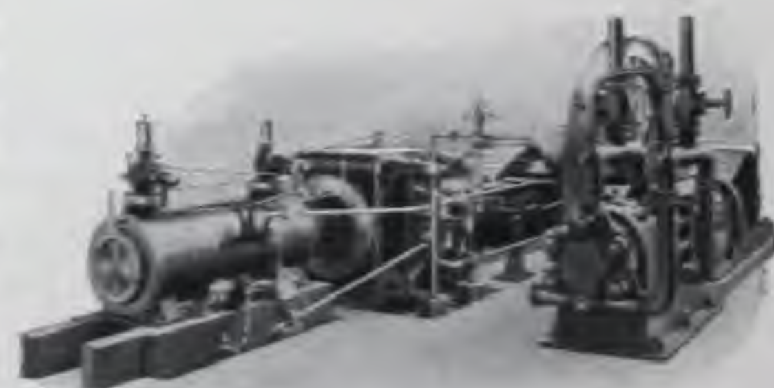
SIMPLE COMPRESSOR, DIRECT CONNECTED TO TANDEM COMPOUND ENGINE WITH HIGH PRESSURE POPPET VALVE CYLINDER AND LOW PRESSURE CORLISS CYLINDER.
