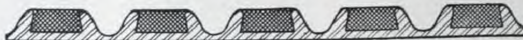
Fig. 3. Cross Section, steel, 5 ribs, 4 inches wide.
