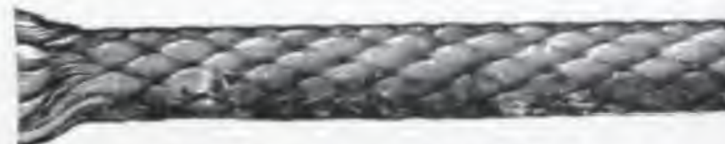
SIZE NO. 10. DIAM. 5-16 IN. About 44 lbs. per doz.; about 27 ft. per lb. Suitable for weights from 30 to 40 lbs. Minimum diam. of pulley allowable, 2 1/2 in.
