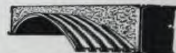
CONCRETE APPLIED TO CURVED PLATE LAID BETWEEN BEAMS.
