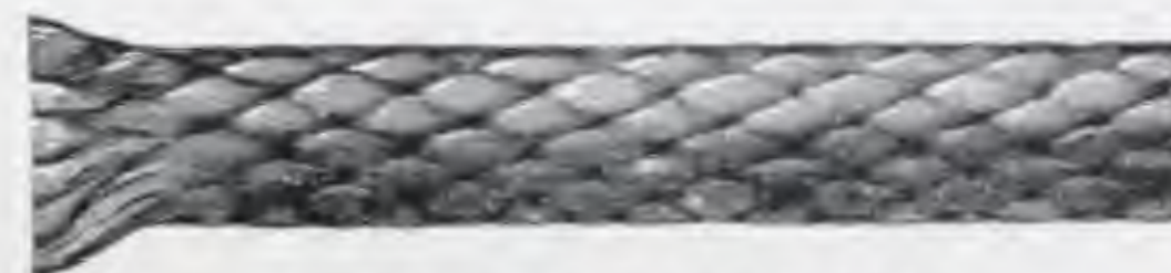
SIZE NO. 12. DIAM. 3/8 IN. About 60 lbs. per doz.; about 20 ft. per lb. Suitable for weights from 40 to 50 lbs. Minimum diam. of pulley allowable, 3 in.
