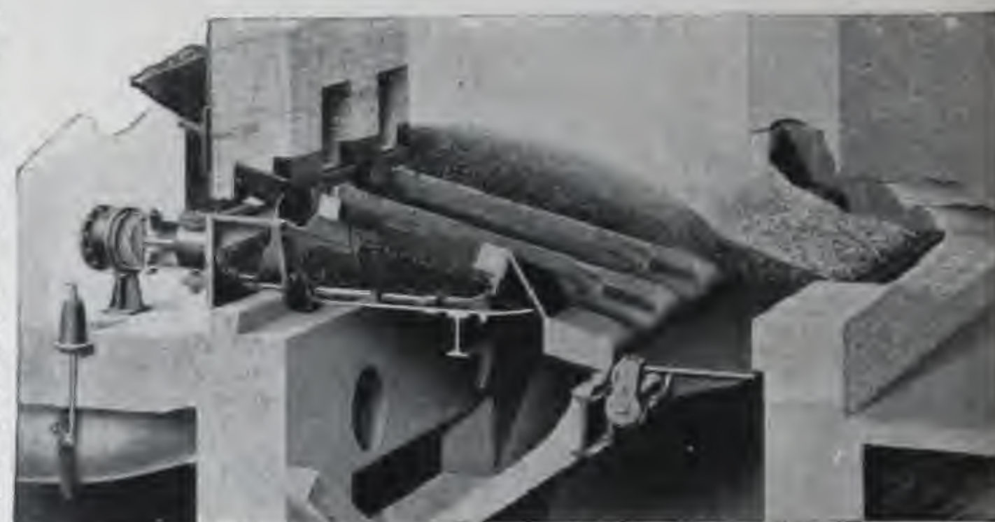
SECTIONAL VIEW THROUGH JONES "A-C" STOKER, SHOWING COUNTER BALANCED DUMP PLATE IN POSITION.
