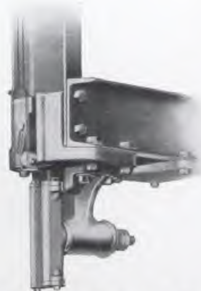
ENLARGED VIEW SHOWING ROLL GRIP SAFETY DEVICE.
