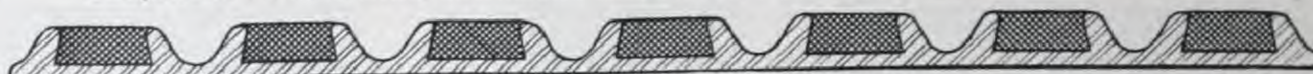
Fig. 1. Cross Section, Steel, 7 ribs, 6 inches wide.
