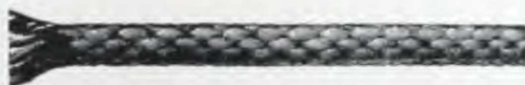
SIZE NO. 6. DIAM. 3-16 IN. About 18 lbs. per doz.; about 66 ft. per lb. Suitable for weights of less than 5 lbs. Minimum diam. of pulley allowable, 1 1/2 in.
