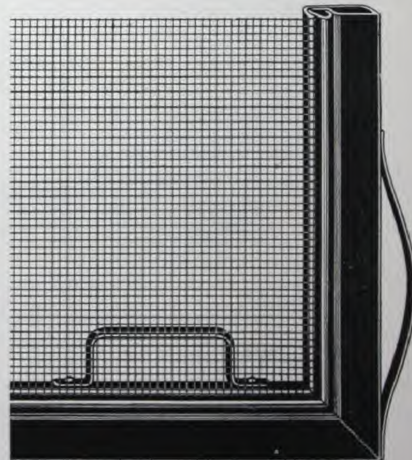
CORNER SECTION SHOWING LIFT AND SIDE SPRING.
