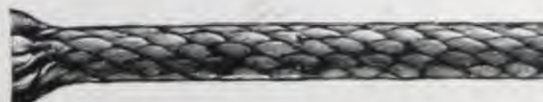
SIZE NO. 8. DIAM. 1/4 IN. About 27 lbs. per doz.; about 44 ft. per lb. Suitable for weights from 12 to 20 lbs. Minimum diam. of pulley allowable, 2 in.
