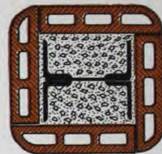
DETAILS OF TYPICAL NATCO COLUMN COVERING.
