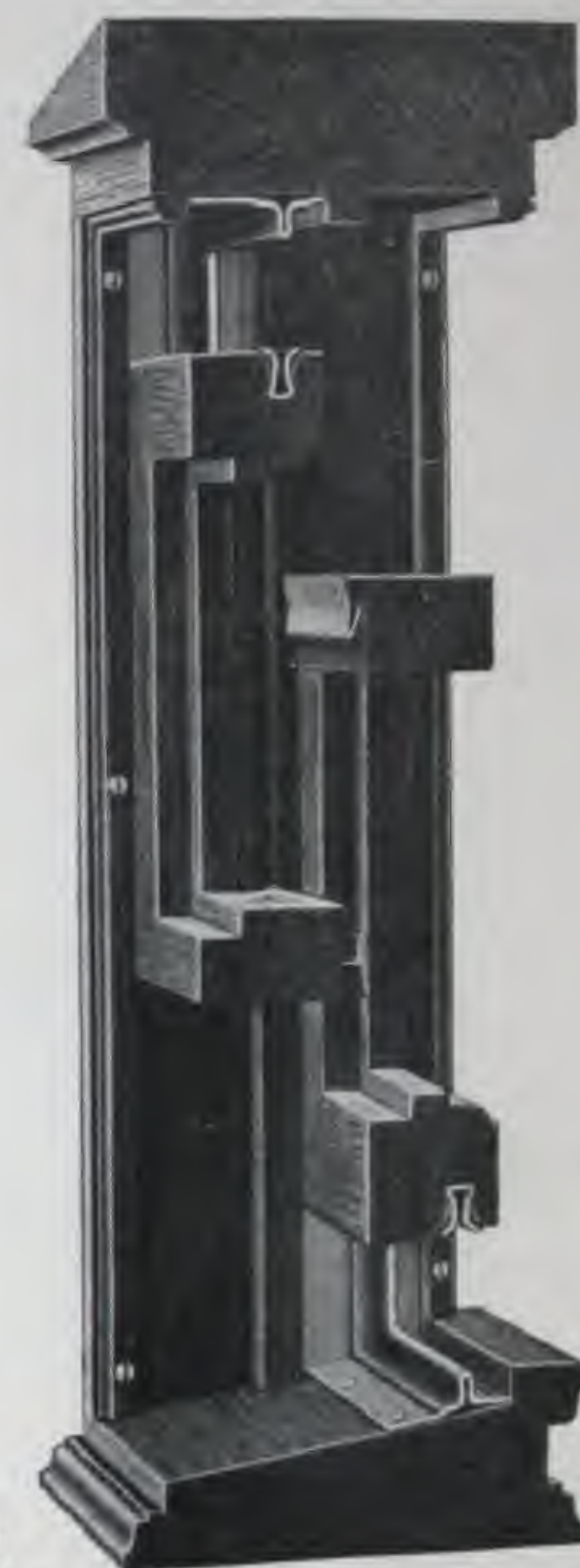
SECTIONAL VIEW SHOWING COMPLETE WEATHER STRIP EQUIPMENT FOR DOUBLE HUNG WINDOW.
