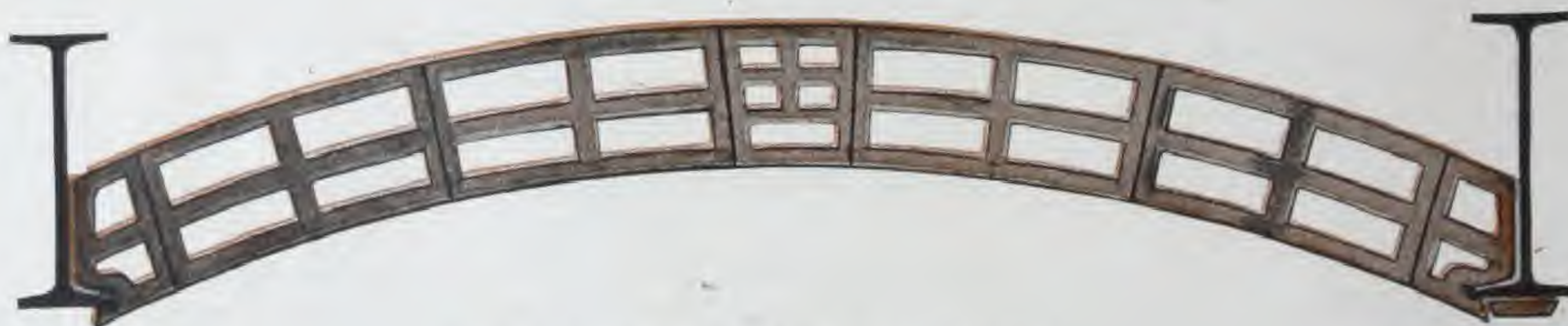
Section Showing Style of Skewbacks and Keys.
