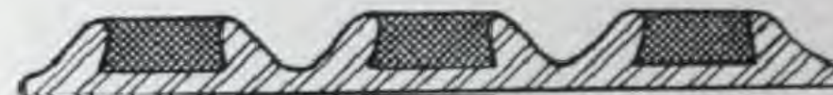
Fig. 6. Cross Section, steel, 3 ribs, 2 1/2 inches wide.
