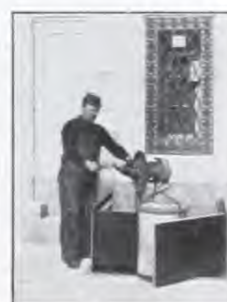
Swinging hoisting head to deposit can on sidewalk, pushes gate open.
