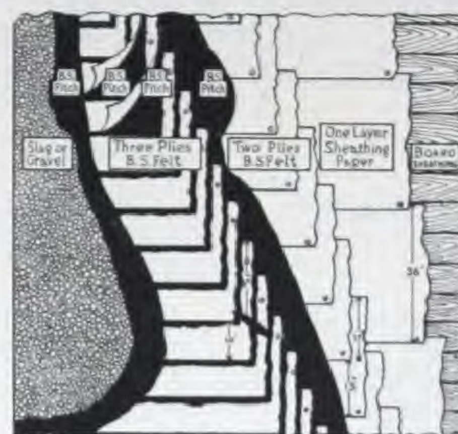
DIAGRAM SHOWING BARRETT SPECIFICATION TYPE "AA" ROOF OVER BOARDS. BONDED FOR 20 YEARS.
