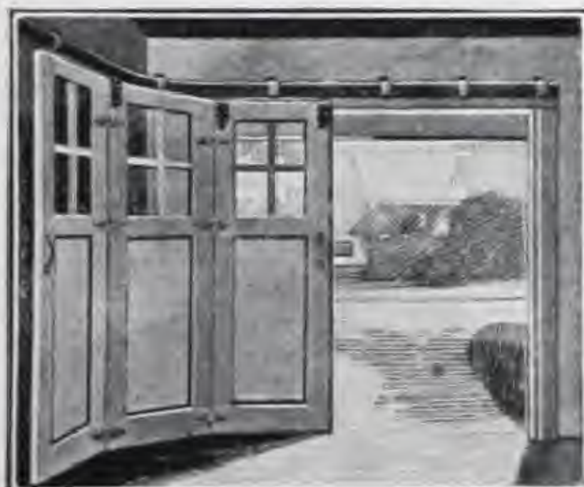
THREE-DOOR TANDEM. Two doors are hung on hangers, the third door is hinged to the middle door and is used as a passage door. Flat track for cheap work, trolley track for good work.
