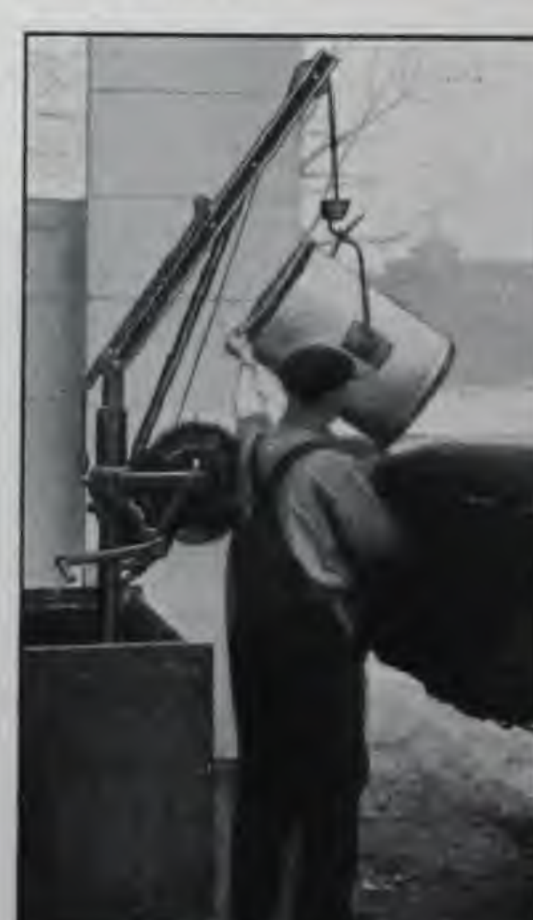
FIG. 5. MODEL B: EMPTYING CAN INTO WAGON. HOISTING HEAD REVOLVES ON BALL-BEARINGS.
