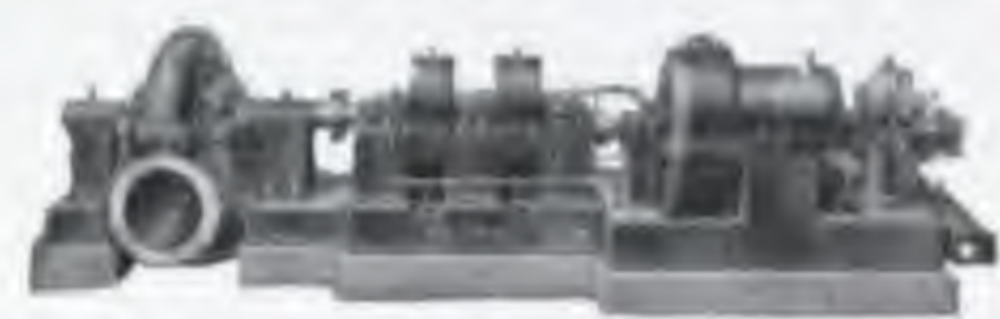
GEARED-TURBINE-DRIVEN CENTRIFUGAL PUMP; 30,000,000 IMP. GAL. PER DAY AGAINST 210 FT. HEAD. INSTALLED AT MONTREAL WATER WORKS.
