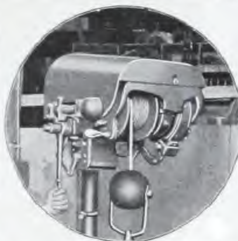
FIG. 7. Close-up view of hoisting head of Model E Hoist, showing hand-lever which controls raising and lowering operations of the hoist.
