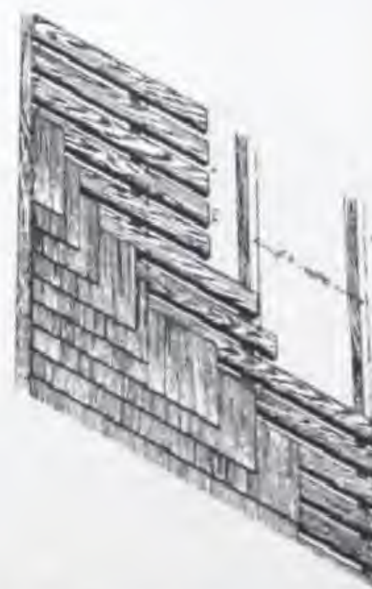
DIAGRAM ILLUSTRATING PARAGRAPH ON SPECIFICATIONS FOR LAYING SHINGLES.
