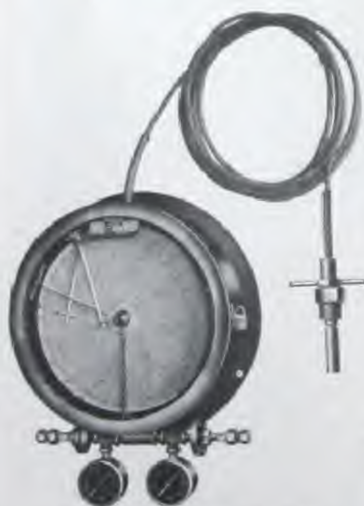
AUTOMATIC TEMPERATURE RECORDER-CONTROLLER. Will operate valves from \frac{1}{4} to 12 in., and on temperatures from -25^{\circ} to +1000^{\circ} Fahr. Set lever with crossarm at required temperature, and this temperature will be maintained automatically until setting is changed.
