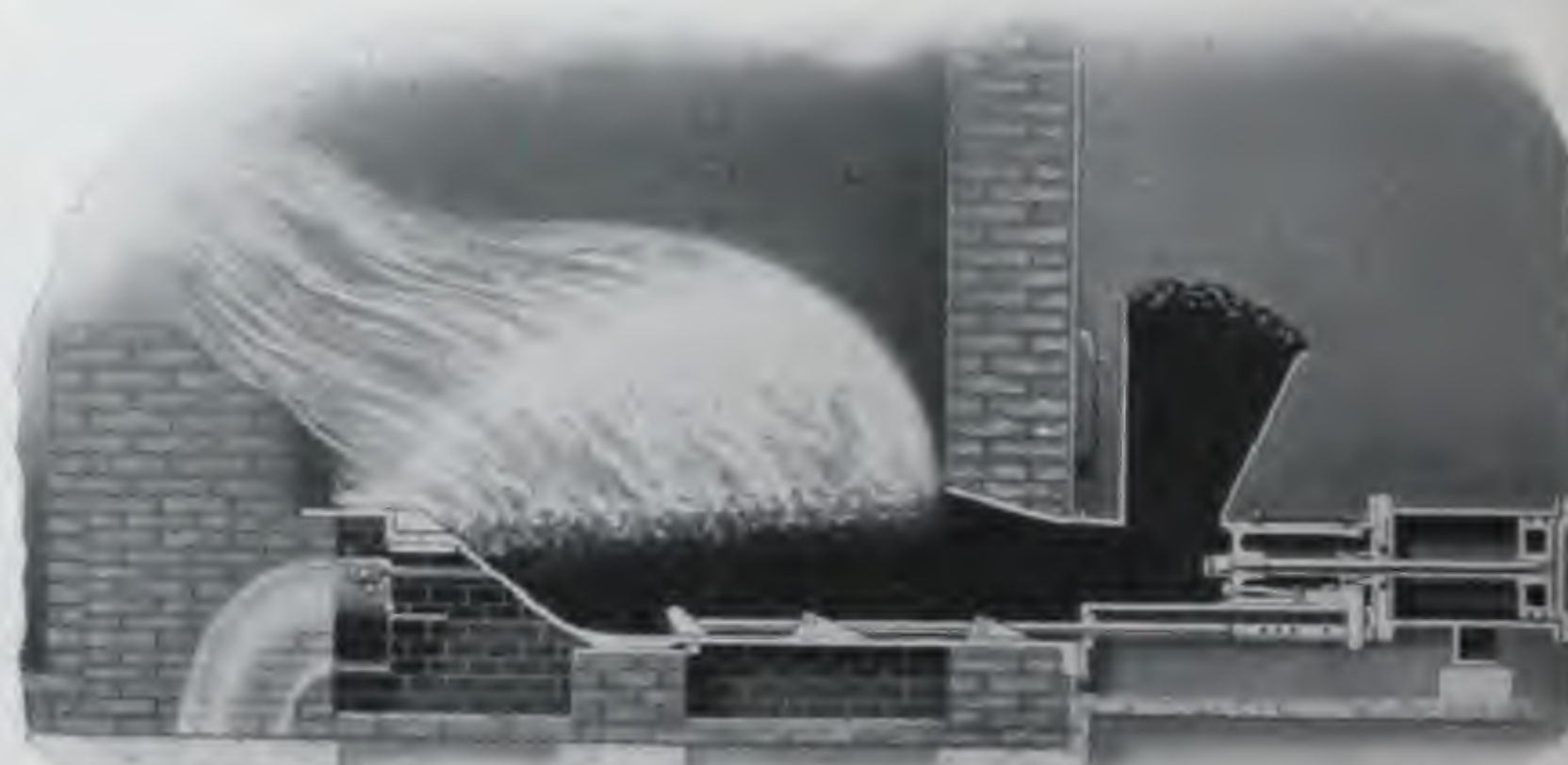
JONES "STANDARD" STOKER—SECTIONAL VIEW.
