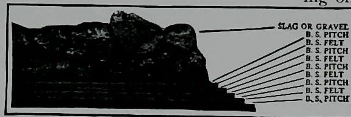
Barrett Specification Roofing
