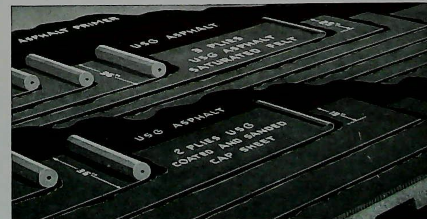
USG 20-Year Bonded Built-up Roof
