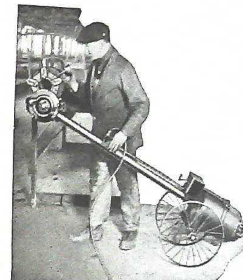
Threading 4-inch Pipe with a Toledo No. 2 Tool Operated by Power Drive
