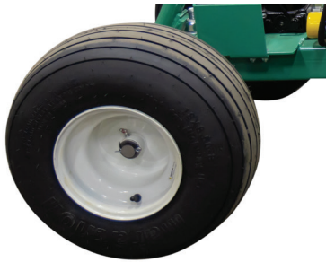
Large smooth air filled tires provide stability and spread surface load.
