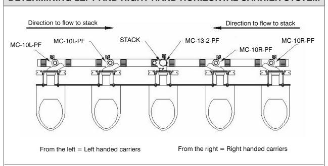
From the perspective of facing the vertical stack, if the toilets are to the left of you, a left handed carrier is required. If the toilets are to the right of you, a right handed carrier is required.
