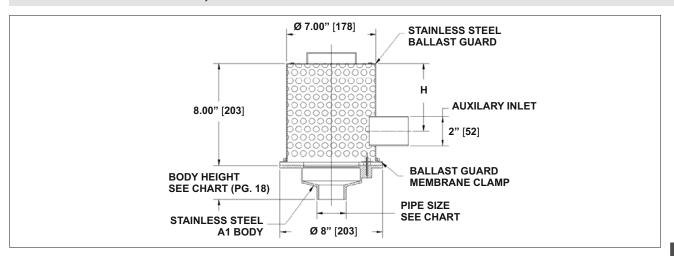
**Description:** MIFAB R1100-28-G8H-AI green roof drain with 8" diameter, cast stainless steel A1 body with 2", 3" or 4" no hub bottom outlet connection, stainless steel membrane clamp, 8" high stainless steel secured ballast guard with auxiliary inlet and removable perforated lid with lift handle.
