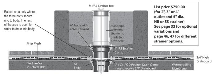
Typically used in planters which are integrated into various locations across the podium. Planters require a secondary concrete pour - over the podium's primary drainage membrane.
