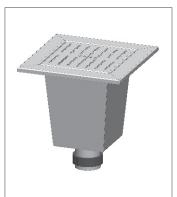
Description: MIFAB FS2000 Series of Type 304 stainless steel floor sink replacement liner for 12" x 12" x 10" deep floor sinks. Manufactured with internal pipe gasket seal and light duty slotted loose set grate and aluminum dome strainer.
