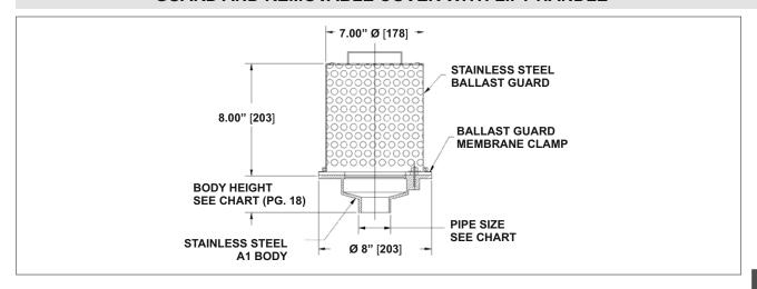
**Description:** MIFAB R1100-28-G8H green roof drain with 8" diameter, cast stainless steel A1 body with 2", 3" or 4" no hub bottom outlet connection, stainless steel membrane clamp, 8" high secured stainless steel ballast guard and removable perforated lid with lift handle.
