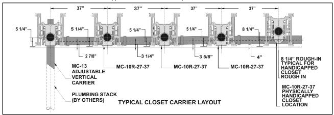
Up to a maximum of ten fixtures may be installed on either side of the stack fitting provided that the waste drain piping is pitched 1/8" per foot.
