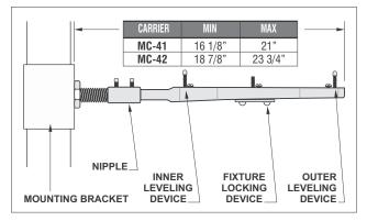
**NOTE:** Minimum and maximum dimensions are front of mounting bracket to the end of the concealed arm. The outermost leveler position is 3/4" from the end of the arm
