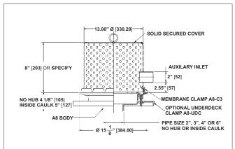
**Description:** MIFAB R1200-JD-M-G8H-Al large green roof drain with 15" diameter, lacquered cast iron A8 body with combination membrane clamp and gravel guard with 8" high perforated stainless steel ballast guard with 2" auxiliary no hub inlet and secured removable access cover with lift handle.
