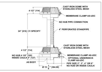
**Description:** MIFAB R1200-JD-W31P24L-R1204-JD large green roof drain with 15" diameter, lacquered cast iron A8 body with combination membrane clamp and gravel guard with low silhouette cast iron, stainless steel mesh covered dome and 24" high perforated PVC standpipe with cast iron body with stainless steel mesh dome on top.
