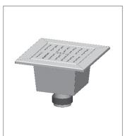
Description: MIFAB FS1980 Series of Type 304 stainless steel floor sink replacement liner for 12" x 12" x 6" deep floor sinks. Manufactured with internal pipe gasket seal and light duty slotted loose set grate and aluminum dome strainer.
