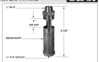
MIFAB's MI-GAP-NPB air gap fitting can be used with MIFAB's MR-500-NPB, M1-500-NPB, M2-500-NPB, MI-TSP-1-NPB, MI-TSP-2-NPB, MI-TSP-3-NPB trap seal primers and MIFAB's MI-DU Series distribution units. The MI-GAP-NPB performs the dual functions of backflow preventer and vacuum breaker. Note: A vertical air gap of twice the connection size is required by code.
