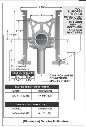
**Note:** 8" tapered thread ABS nipple shipped standard with MC-14 Series carriers. The universal faceplate assembly accepts all nipple variations, rolling thread (-OR), cast iron (-CI) and tapered thread ABS with adjustable horn (-AH). (See page 224).
