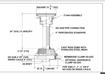
**Description:** MIFAB R1200-JD-W31P24L-F1444 large green roof drain with 15" diameter, lacquered cast iron A8 body with combination membrane clamp and gravel guard with low silhouette cast iron, stainless steel mesh covered dome and 24" high perforated PVC standpipe with cast iron body and 12" x 12" ductile iron strainer on top.
