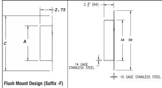
Note: The R1960 and R1960-F models are made to receive PVC, ABS or cast iron pipe inside the "A" dimension. The R1960 models "sleeve" over the pipe sticking out from the wall. The R1960-F models "sleeve" over the pipe that is flush to the wall.
