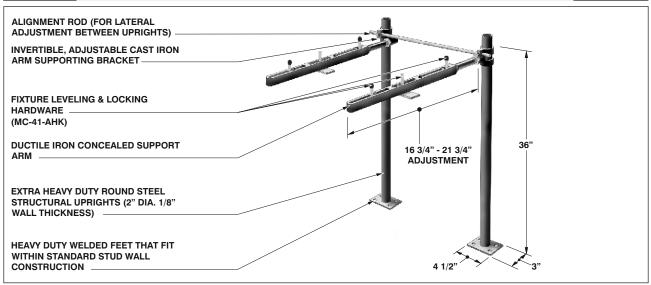
NOTE: Foot supports should be securely anchored to floor with ½" bolts and anchors by others
