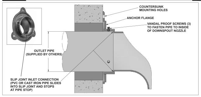
The (slip joint inlet downspout nozzle) performs the same function as the R1940 downspout nozzle. The difference between the two is the method of connecting the pipe to the inlet. With the R1940-SJ, the inlet is machined out. This allows cast iron or PVC pipe to extend past the face of the finished wall and rest against the pipe stop. The pipe is secured to the inside of the R1940-SJ via three vandal proof screws.
