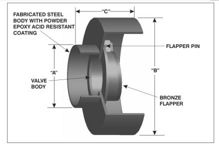
Note: The BV1280 terminal valve is used at the end of sewer lines to prevent backflow into areas that require draining.
