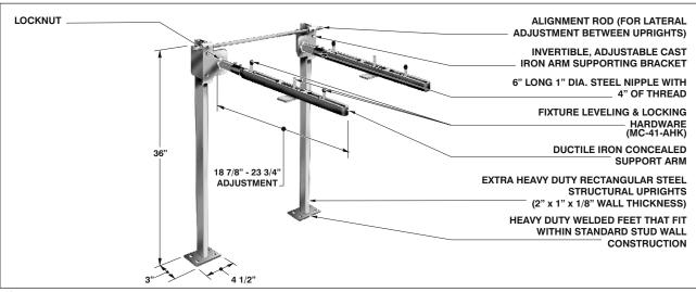
$\textbf{NOTE:} \ \ \text{Foot supports should be securely anchored to floor with } 1 \!\!/\!\!2" \ \ \text{bolts and anchors by others}$
