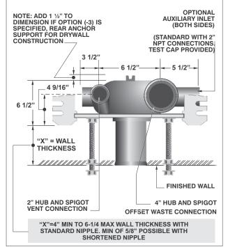
\*MC-15-HS is tested to support a 500 lb. load with the rear anchor support.
