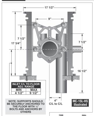
Note: 8" tapered thread ABS nipple shipped standard with MC-15 Series carriers. The universal faceplate assembly accepts all nipple variations, rolling thread (-OR), cast iron (-CI) and tapered thread ABS with adjustable horn (-AH). (See page 224).
