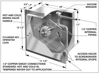
MIFAB Series F1670 water supply control box manufactured from Type 304 stainless steel. Box complete with cylinder key lock. Features single hot and cold mixing valve handle and atmospheric type vacuum breaker with integral screwdriver stops.
