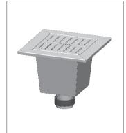
Description: MIFAB FS1990 Series of Type 304 stainless steel floor sink replacement liner for 12" x 12" x 8" deep floor sinks. Manufactured with internal pipe gasket seal and light duty slotted loose set grate and aluminum dome strainer.
