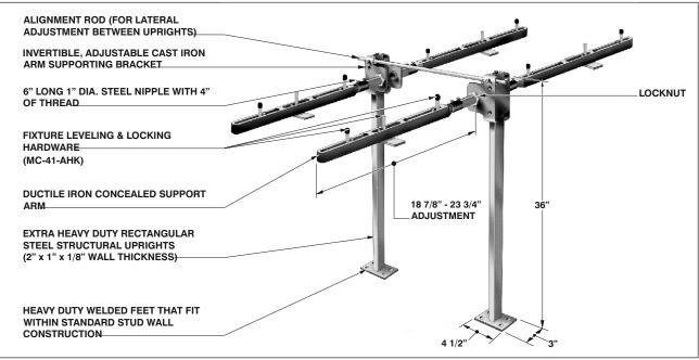
NOTE: Foot supports should be securely anchored to floor with ½" bolts and anchors by others
