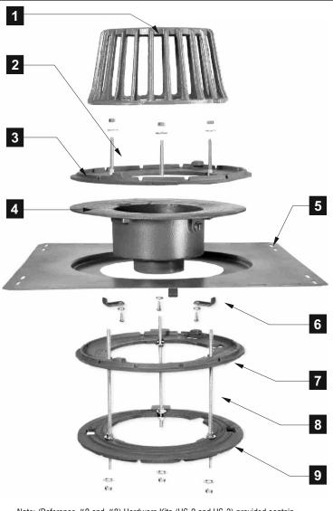
Note: (Reference #2 and #8) Hardware Kits (HS-2 and HS-3) provided contain standard 5/16" all threaded studs. Upon installation, excess rod may be cut to desired length for clean installation.
