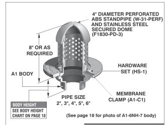
F1830-P PLANTING AREA DRAIN WITH 8" HIGH PERFORATED STANDPIPE AND DOME
