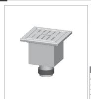
Description: MIFAB FS1970 Series of Type 304 stainless steel floor sink replacement liner for 8" x 8" x 6" deep floor sinks. Manufactured with internal pipe gasket seal and light duty slotted loose set grate and aluminum dome strainer.
