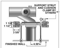
Note: 8" tapered thread ABS nipple shipped standard with MC-10 Series carriers. The universal faceplate assembly accepts all nipple variations, rolling thread (-OR), cast iron (-Cl) and tapered thread ABS with adjustable horn (-AH). (See page 224)
