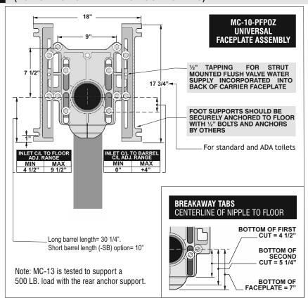
Note: 8" tapered thread ABS nipple shipped standard with MC-13 Series carriers. The universal faceplate assembly accepts all nipple variations, rolling thread (-OR), cast iron (-CI) and tapered thread ABS with adjustable horn (-AH). (See page 224).
