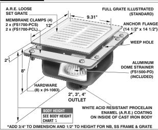
Note: Specify outlet size and connection type. Dome strainer
