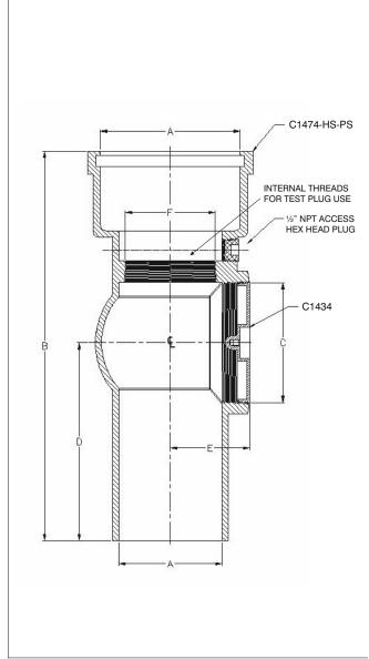
**Function:** The C1470 Series is used in concealed drainage lines where access to the piping is required via a cleanout that per testing of the piping above the plug through the use of internal threads inside of the tee.
