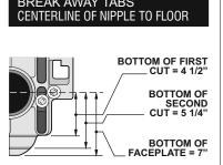
Note: 8" tapered thread ABS nipple shipped standard with MC-10 Series carriers. The universal faceplate assembly accepts all nipple variations, rolling thread (-OR), cast iron (-CI) and tapered thread ABS with adjustable horn (-AH). (See page 224).
