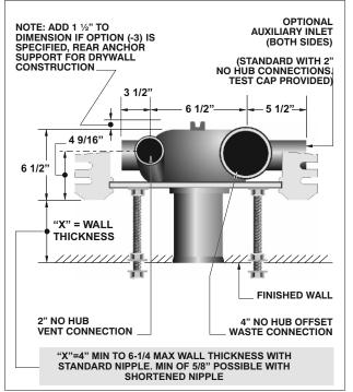
\*MC-15 is tested to support a 500 lb. load with the rear anchor support.
