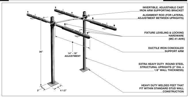
**NOTE:** Foot supports should be securely anchored to floor with  $\frac{1}{2}$ " bolts and anchors by others
