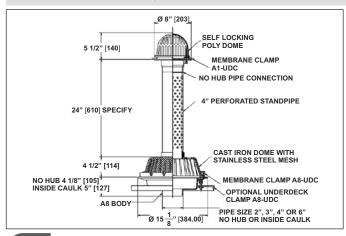
Description: MIFAB R1200-JD-W31P24L-R1104 large green roof drain with 15" diameter, lacquered cast iron A8 body with combination membrane clamp and gravel guard with low silhouette cast iron, stainless steel mesh covered dome and 24" high perforated PVC standpipe with cast iron body and poly dome strainer on top.
