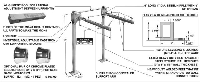
NOTE: Foot supports should be securely anchored to floor with 1/2" bolts and anchors by others
