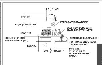
**Description:** MIFAB R1200-JD-W31P6L-WD large green roof drain with 15" diameter, lacquered cast iron A8 body with combination membrane clamp and gravel guard with low silhouette cast iron. stainless steel mesh covered dome and 6" high perforated PVC standpipe.
