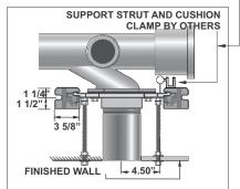
Note: 8" tapered thread ABS nipple shipped standard with MC-10 Series carriers. The universal faceplate assembly accepts all nipple variations, rolling thread (-OR), cast iron (-CI) and tapered thread ABS with adjustable horn (-AH). (See page 224)
