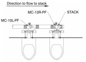
From the perspective of facing the vertical stack, if the open inlet is to the left of you, you have a left handed carrier. If the open inlet is to the right of you, you have a right handed carrier.
