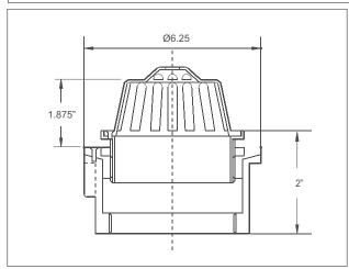
NOTE: Any F1100 Series strainer can be used in place of the K dome strainer. See pages 46 and 47 for selection and prices.
