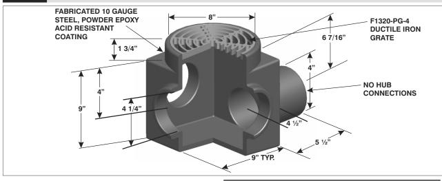
Note: The function of the BV1290 is to provide a sump with multiple inlets that the foundation drain lines connect to.
