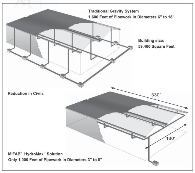
The MIFAB HYDROMAX siphonic roof drain system is designed to have high flow capacities while minimizing ponding. Mifab's unique system prevents air ingress into the pipework, combined with a hydraulically designed pipe system, allows for high performance siphonic flows. The advanced Mifab® HydroTechnic™ online analytical design calculation software program which has been independently tested for full compliance with ASPE/ANSI 45, provides calculations for optimum system efficiency.
