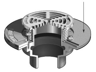
Specify MIFAB'S floor drains with heavy duty stainless steel strainers **FOR THE SAME PRICE** as conventional floor drains with membrane clamps and light duty nickel bronze strainers.
