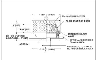
**Description:** MIFAB R1200-JD-M-G5H large green roof drain with 15" diameter, lacquered cast iron A8 body with combination membrane clamp and gravel guard with low silhouette cast iron dome and 5" high perforated stainless steel ballast guard with secured removable access cover and lift handle.
