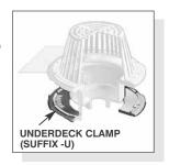
against the bottom of the deck and drawn tightly in place with hardware provided. This in effect sandwiches the deck into a positive union with the drain. Thus secured into place, the roof drain becomes an integral component of the deck with assurance of installation stability and optimum performance in its role as entrance terminal of the roof drainage system. **Specify Suffix –U**
