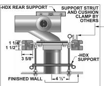
Note: 8" tapered thread ABS nipple shipped standard with MC-10 Series carriers. The universal faceplate assembly accepts all nipple variations, rolling thread (-OR), cast iron (-CI) and tapered thread ABS with adjustable horn (-AH). (See page 224).
