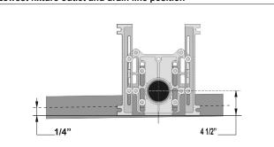
Highest fixture outlet and drain line position
