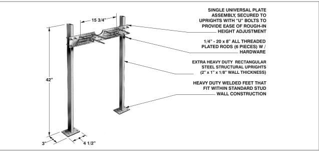
**NOTE:** Foot supports should be securely anchored to floor with  $\frac{1}{2}$ " bolts and anchors by others
