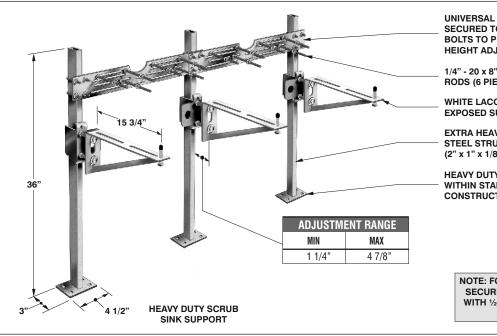
UNIVERSAL PLATE ASSEMBLY, SECURED TO UPRIGHTS WITH "U" BOLTS TO PROVIDE EASE OF ROUGH-IN HEIGHT ADJUSTMENT
