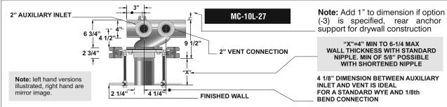
Note: 8" tapered thread ABS nipple shipped standard with MC-10 Series carriers. The universal faceplate assembly accepts all nipple variations, rolling thread (-OR), cast iron (-CI) and tapered thread ABS with adjustable horn (-AH). (See page 224).
