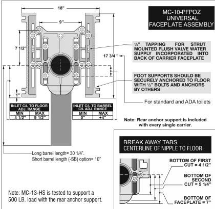
Note: 8" tapered thread ABS nipple shipped standard with MC-13 Series carriers. The universal faceplate assembly accepts all nipple variations, rolling thread (-OR), cast iron (-CI) and tapered thread ABS with adjustable horn (-AH). (See page 224).
