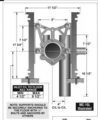
Note: 8" tapered thread ABS nipple shipped standard with MC-15 Series carriers. The universal faceplate assembly accepts all nipple variations, rolling thread (-OR), cast iron (-Cl) and tapered thread ABS with adjustable horn (-AH). (See page 224).
