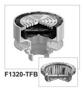
True-fit bucket design ensures bucket replacement after cleaning since the top grate cannot be inserted unless the bucket is in place because the grate is set into the bucket and the bucket suspends within the top assembly. Integral with F1320-TFB, F1340-TFB and F1360-TFB area drains.
