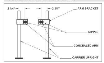
The center of the concealed arm nipple is 2 1/4" offset from center line of the uprights. It is imperative that this offset be accommodated when locating the position of the upright before it is lag bolted to the floor slab!
