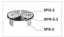
The SPR-5-3(-1 for NB) is used with 5-1 and 5-3 strainers to increase the height of the strainer to match discrepancies in the finished floor grade. Any number of rings can be added on top of each other. Each ring adds 3/8"of height. Simply remove the grate, place the SPR-5-3(-1 for NB) into the cast in place shank, and then screw the grate into the ring. Longer bolts are provided by MIFAB. The vertical height of the strainer can be adjusted after the drain is poured in place.
