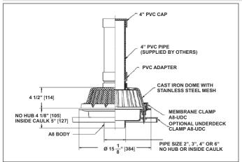
**Description:** MIFAB R1200-JD-W30 large green roof drain with 15" diameter, lacquered cast iron A8 body with combination membrane clamp and gravel guard with low silhouette cast iron, stainless steel mesh covered dome and top PVC cap.
