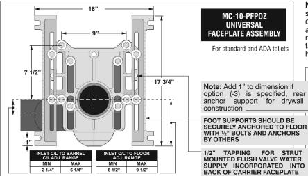
Note: 8" tapered thread ABS nipple shipped standard with MC-10 Series carriers. The universal faceplate assembly accepts all nipple variations, rolling thread (-OR), cast iron (-CI) and tapered thread ABS with adjustable horn (-AH). (See page 224).
