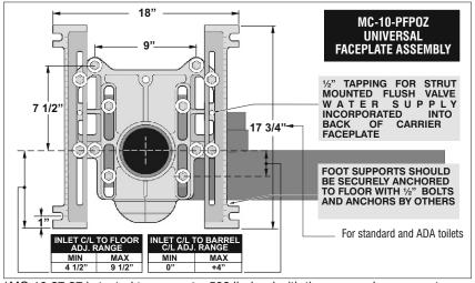
Note: 8" tapered thread ABS nipple shipped standard with MC-10 Series carriers. The universal faceplate assembly accepts all nipple variations, rolling thread (-OR), cast iron (-CI) and tapered thread ABS with adjustable horn (-AH). (See page 224).
