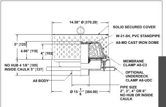
**Description:** MIFAB R1200-JD-M-G5H-W31H4 large green roof drain with 15" diameter, lacquered cast iron A8 body with combination membrane clamp and gravel guard with low silhouette cast iron dome, ABS standpipe, 5" high perforated stainless steel ballast guard with secured removable access cover and lift handle.
