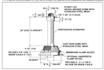
Description: MIFAB R1200-JD-W31P24L-R1404T-1-83 large green roof drain with 15" diameter, lacquered cast iron A8 body with combination membrane clamp and gravel guard with low silhouette cast iron, stainless steel mesh covered dome and 24" high perforated PVC standpipe with cast iron body and nickel bronze strainer with stainless steel mesh dome on top.
