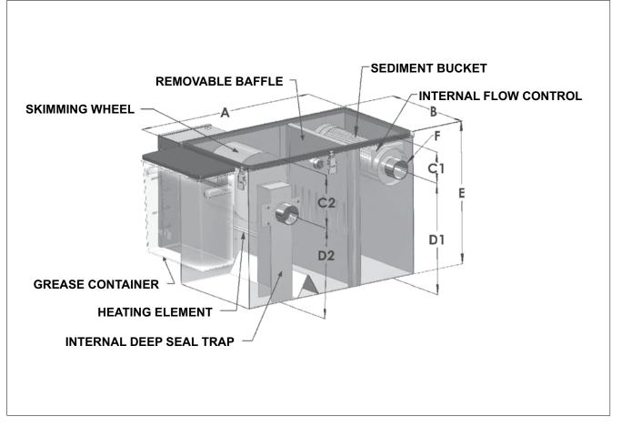
The MI-G-AD Series is an automatic recovery grease interceptor that is self cleaning and requires minimal maintenance. The unit intercepts solids with an internal sediment bucket and extracts free floating oil and grease from the unit automatically into a separate holding compartment.
