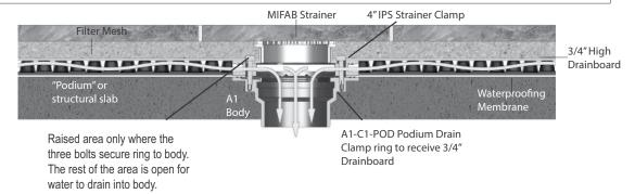
Note: This is the typical installation for the below paver podium system. Check with contractor for installation required for each jobsite.
