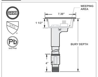
The wetted surface contacted by consumable water contains less than one quarter of one percent (0.25%) of lead by weight.
