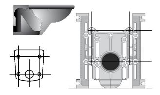
BLOWOUT WATER CLOSETS use a direct jet stream for bowl evacuation. This type of flushing action is rapid and forceful and primarily used in heavy duty installations such as stadiums and terminals. Due to this powerful flushing, the blowout water closet is noisier in operation than the siphon jet. The blowout closet mounts to the wall with three mounting studs. NOTE: It is highly unadvisable to mount Blow-out type water closets in a "Back to Back" type installation.
