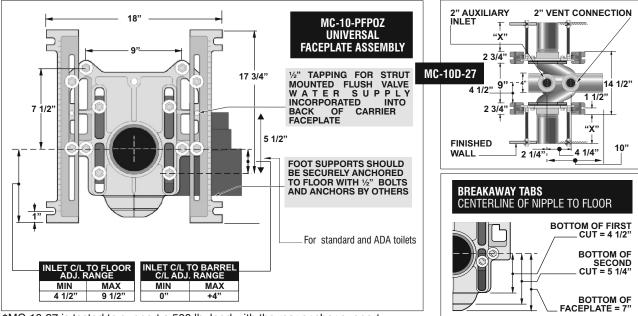
\*MC-10-27 is tested to support a 500 lb. load with the rear anchor support.
